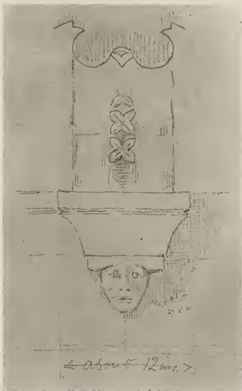
Fig. 213. Corbel, Impost and Vault Rib of Rotunda, Templar's Church, Loon.
