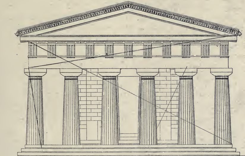
187. Temple of Poseidon at Pæstum. The diagonals indicate the approximate relations between the parts.
