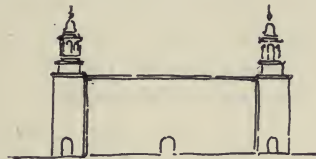
217. Showing what might be done with 215 if the projection of the flanking masses could be reduced.
