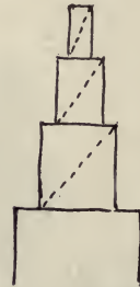
171. Correct method of proportioning a storied tower.
