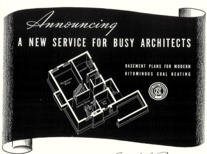
The fundamental principles of designing basements for modern Bituminous Coal heating can be combined into this simple statement: Keep the driveway, coal storage and heating units as close together as possible.
