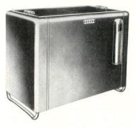
The new Norge beverage coolers are of immersion type, powered with a Rollator compressor. Cabinet is constructed of anti-rust treated furniture steel, built around and supported by heavy, all-steel, welded center and bottom frames of battleship construction. High baked enamel is used for exterior finish in vermilion red
