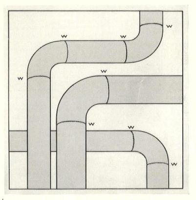
The welds, "W", are smooth inside, and practically flush with the pipe wall outside. Consider the simplicity of this group of welded connections in comparison with the joints made by any other method.
