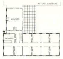
Dormitory for small country college adjacent to and to harmonize with an existing building of pseudo-colonial style. Note: use of stock sash, retaining vertical muntins; exterior surface stuccoed and painted to match existing building; special cornice developed to match; one story lounge, at lower level, utilizing panels set horizontally BELOW others, giving 12' ceiling height
