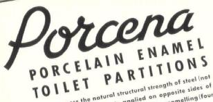
Porcena Panels possess the natural structural strength of steel (not one sheet but two 16 gauge sheets applied on opposite sides of sound-deadening core) strengthened by porcelain enamelling(four layers) which provides a non-porous, flint-hard glass-smooth surface that is positively impervious to odors, acids, and moisture.
