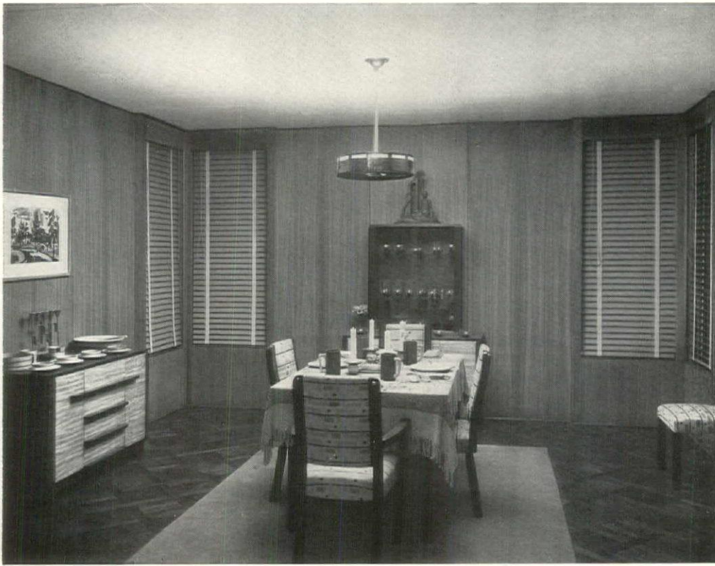
Dining rooms require even general illumination with a special emphasis of local light upon the table. Above, one ceiling fixture supplies both. Opposite page: upper left, general illumination from indirect torcheres; upper right, general illumination from well shaded ceiling candelabra and wall fixtures.
