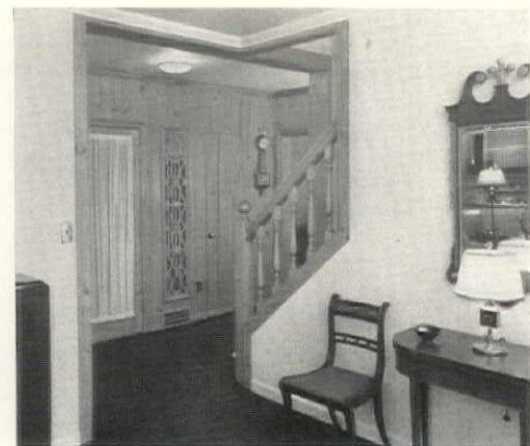
At left, general exterior illumination of an entrance is better than small spotty lights. Center, a small ceiling bowl lights both entrance hall and stairs. Right, closet is lit by ceiling fixture. Jamb light helps mirror viewing.
