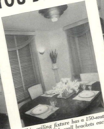
This breakfast room is lighted with an inner diffusing bowl fixture containing a 100-watt lamp.
