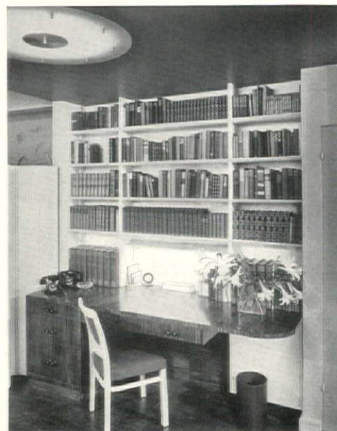
Local lighting in limited space at work area; general illumination provided by ceiling fixture.
