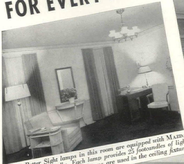
This ceiling fixture has a 150-watt lamp. Four side-wall brackets each contain a 40-watt lamp.
