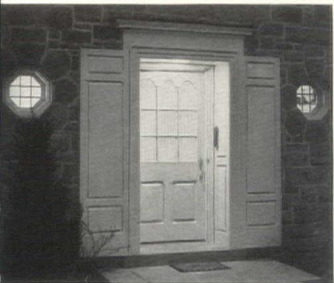
At left, general exterior illumination of an entrance is better than small spotty lights. Center, a small ceiling bowl lights both entrance hall and stairs. Right, closet is lit by ceiling fixture. Jamb light helps mirror viewing.
