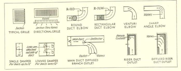
Fig. 8. Details of warm air heating and air conditioning ducts and outlets
