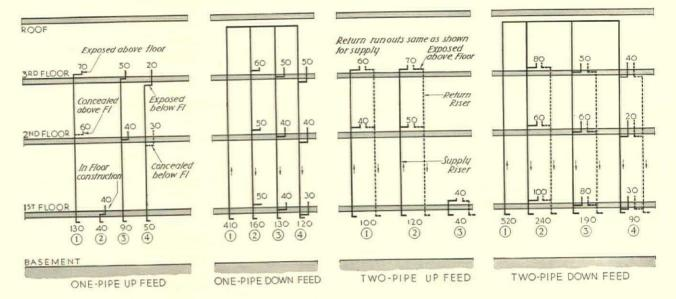
Fig. 5. Typical riser diagrams. Capacity of connected radiation is indicated by figures at radiator connections (in EDR). Total radiation connected by each riser is noted at foot of riser. Each riser should be numbered for reference purposes
