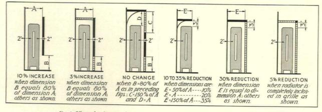
Fig. 6. Effect of radiator enclosures compared to heat emitted by a free standing radiator
