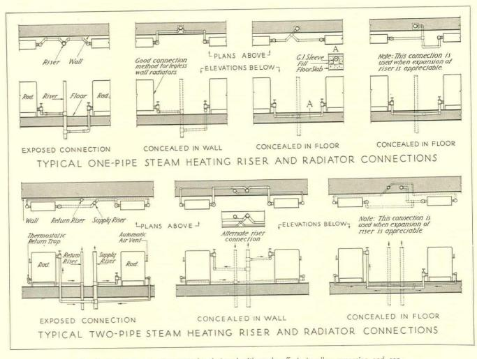
Fig. 7. Radiator connections must be designed with angle offsets to allow expansion and contraction of risers and runouts without disturbing radiation or stressing pipe or structural members
