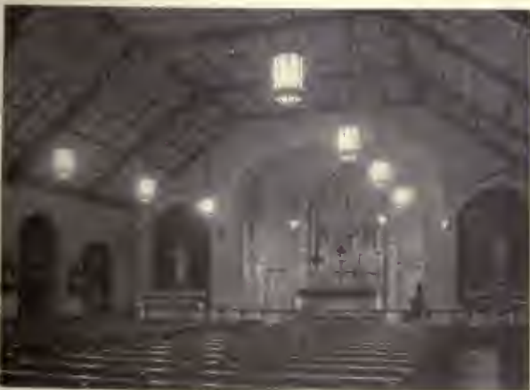
Our Lady of Guadalupe Church, Brooklyn, N. Y., with diffused lights. When fixtures are hung equidistant from surfaces to be illuminated, the maximum light efficiency is obtained without impairing the decorative scheme
