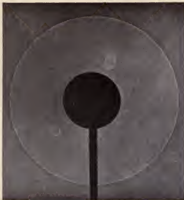
Fig. 1. Sound Impulse generated by the snap of an electric spark
