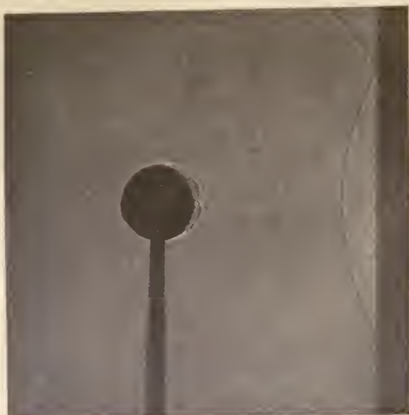
Fig. 2. Reflection at a hard impervious surface
