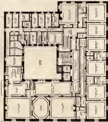
TYPICAL UPPER FLOOR PLAN SHOWING SINGLE APARTMENT ON LEFT AND PART OF DUPLEX ON RIGHT
