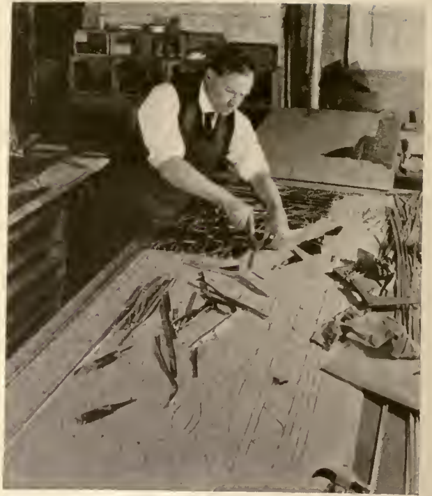
Fig. 8. "Leading-Up" or Glazing The pieces assembled on the cut-line Drawing
