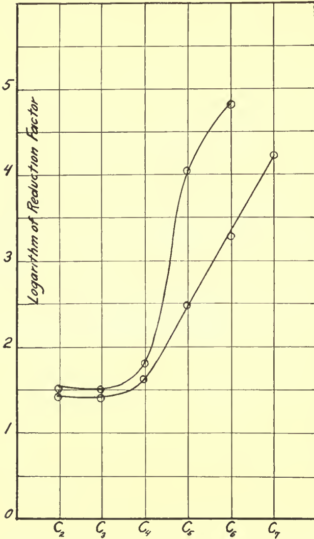
Figure 5. Reduction of Intensity of Sound transmitted by three doublets of Hair Felt and Paper. Upper curve represents the measured values; lower curve as computed
