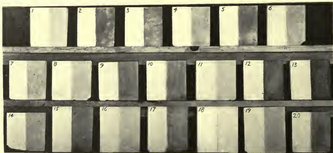
Appearance of treated stone in waterproofing tests. Some are changed less by the treatment than by a year of exposure to soot and smoke.
