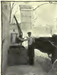
Operator raises the filled can without leaving sidewalk. Then hoisting head
