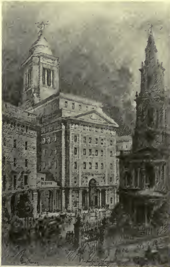
PERSPECTIVE WITH MODIFIED STUDY OF TOWER AND STREET FRONT OF BUILDING RAISED ONE STORY ABOVE LEGAL HEIGHT WHICH WAS PERMITTED BY SPECIAL ACT OF LONDON COUNTY COUNCIL BECAUSE OF THE "ARCHITECTURAL" NECESSITY OF A DOMINATING CENTRAL MOTIVE IN A FAÇADE SO LONG
