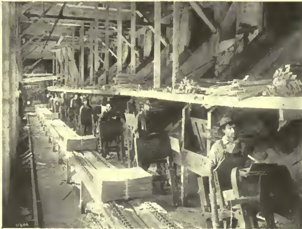
FIG. 6. THE SHINGLES ARE BUNDLED AND CONVEYED TO FREIGHT CARS
