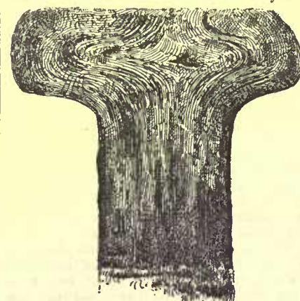
Magnified sectional view of the head of a cut nail showing the distortion of the fibres of the iron occasioned by upsetting during manufacture.
