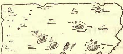
Fig. 17.—Tin Pipe taken from Cambridge, Mass., corroded.
