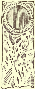
Fig. 13.—Trap-top corroded by Mortar or Slaked Lime.
