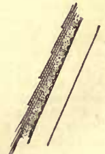
Fig. 10. Slate fastened to corrugated sheet-iron by wrought-iron countersunk pins. Slate is also bedded in a layer of cement applied to corrugated iron.
