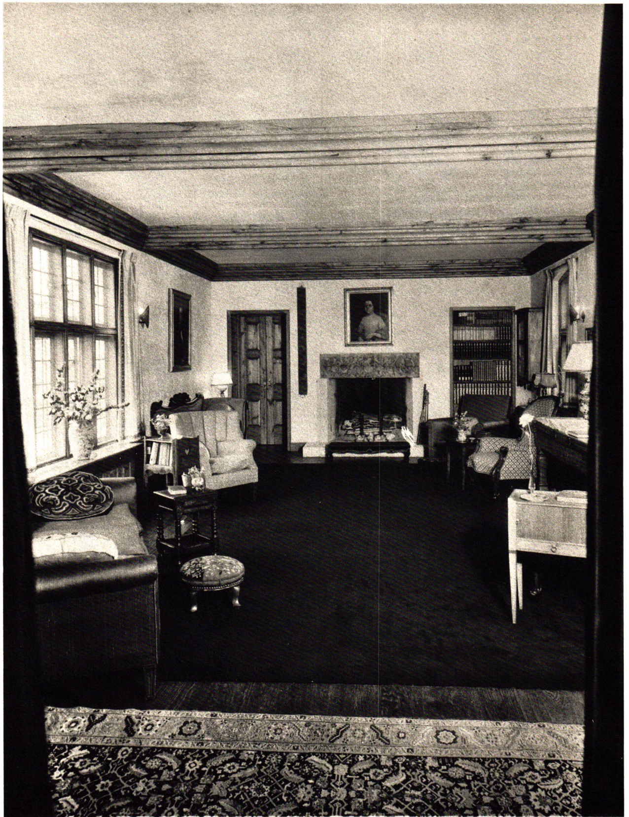
Looking into the living-room from the upper level of the hall. The carved oak lintel and limestone jambs frame the fireplace and its raised hearth. Here the ceiling beams are moulded oak. The walls and ceiling are of smooth sand plaster. Wide oak planks are used for the flooring
