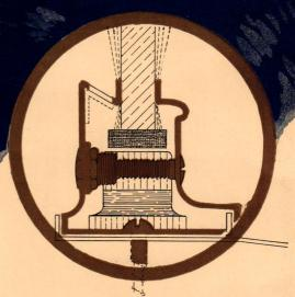
Two of the outstanding features of Kawneer Solid Copper Store Fronts are Strength and Resiliency. Maximum strength is obtained through the use of solid copper in sturdy construction; resiliency, by the spring-like grip by which the plate glass is held securely in position, enabling shock and strain to vibrate out through the edge of the glass.
