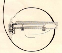
Cross section, showing the Tepeco concealed bracket and how it is secured to lavatory. Note the adjustment provided in the bolts locking the lavatory to the brackets, which also provides for the leveling of the lavatory. It may be installed to set the lavatory at any desired height from the floor. There is a Tepeco bracket for every form of wall connection.
