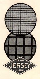
In the upper circle is shown an unretouched photograph, actual size, of Copper Screen Cloth (heavy grade) made by The New Jersey Wire Cloth Company, which has been subjected to the action of salt air for more than twelve years.
