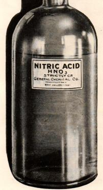
Drop a piece of lead, brass, steel, cast or wrought iron into a beaker of Nitric Acid, and you will see the metal attacked *instantly*, and in a short time entirely destroyed.
