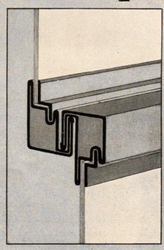
The workability of Ambrac Metal is well illustrated by this view of some of the shapes which it must assume in giving weather-tightness to
