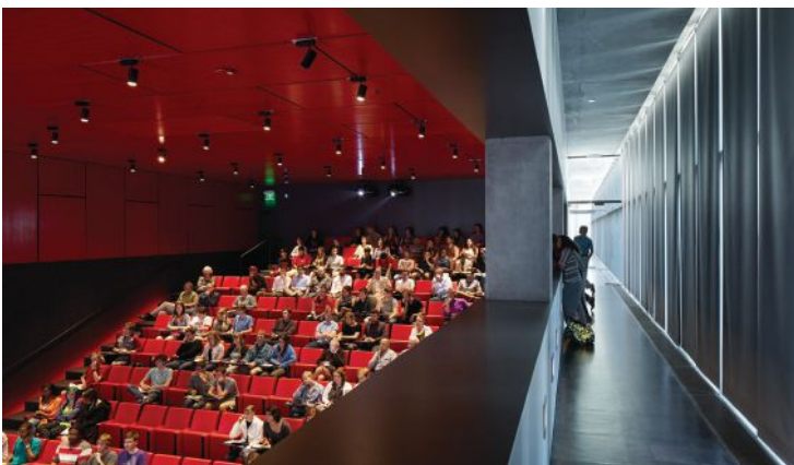
The corridor that runs from the east entrance is lit by a series of vitrines that are used to display student work (top left). The vitrines are illuminated with 32W T8 fluorescent fixtures. The interior of the cases house asymmetric LED wallwashers at 9W-per-linear-foot. In the 200-seat auditorium (left), the lighting is set on separately controlled layers to meet the needs of the space. The LED ceiling downlights are dimmable and shades along the corridor window wall can be drawn for projection presentations and films. In the exhibition gallery, recessed lensed 26W CFL downlights are used (above). In the studios (opposite), natural light is balanced with 32W T8 direct-indirect pendant fixtures overhead and additional tasklighting at the workplane.
