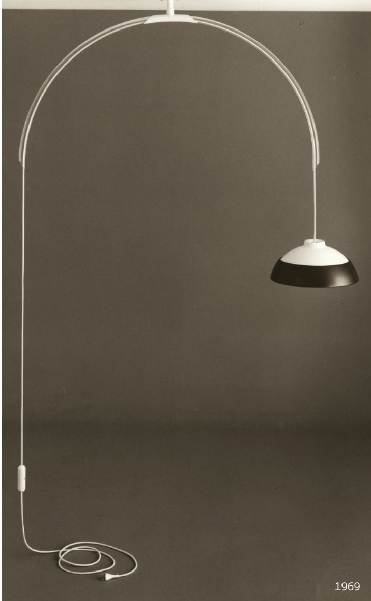
Sinfatti's design for Model 2129 (this page) originally used an E27 100W incandescent lamp. The new version uses 15W 2700K LEDs and positions the heat sink, the circuit board, and the diffuser inside, and at the top of, the shade. For the two floor lamps—Model 1063 (opposite, top) and Model 1095 (opposite, bottom)—the switch to LED was also an easy transition, as the existing power supplies were re-engineered to accommodate the LED drivers.
