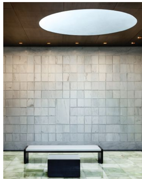
A contemplative but soothing atmosphere is created by the abundance of natural light that permeates the interiors. Each room has a slightly different feel due to the variations in shape and position of the skylights. In one north-facing columbarium, accented with green onyx flooring (above), an oculus functions as the primary luminaire, while MR16 wallwashers provide the balance of electric light.
