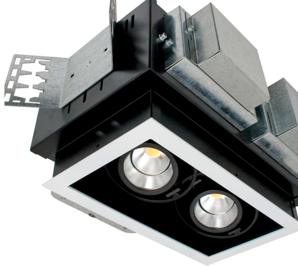
Pluris Series, Intense Lighting • The Pluris series, an LED multilight, features lamp holders that are adjustable 365-degree horizontal and 45-degree vertical for a range of narrow-flood, flood, and wide-flood beam spreads. Three color temperatures are available (3000K, 3500K, and 4100K), as are two lumen packages (650 lumens with an input power of 15W, and 900 lumens for 17.8W). For ease of use and maintenance, all components are accessible from below the ceiling. One-, two-, three-, and four-lamp configurations are available. Dimming to 10 percent output is also possible. intenseighting.com • Circle 152
