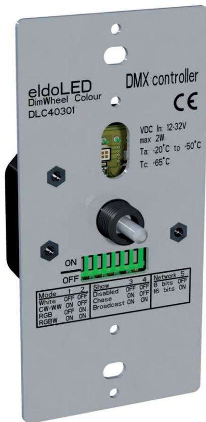
DimWheel Series, EldoLED • This is a one-button DMX controller that sets dim level, color, and show for LED drivers and DMX compatible luminaires. It works with most dimmer face plates and meets U.S., U.K., and European Union wall-box size requirements. The one-channel mode dims the light and turns it off and on for general white LED lighting applications. A two-channel mode allows for mixing of warm- and cool-white light. For static and dynamic full-color applications (RGB and RGB/A) there are three- and four-channel modes. The U.S. model measures 2 inches wide by 4.12 inches tall. eldoled.com • Circle 300
