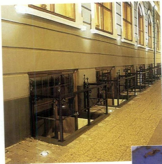
FIBER OPTICS ARE PROVIDING THE UPLIGHTS ON THIS BUILDING. WITH A TOTAL EQUIPMENT COST OF LESS THAN $400 PER FIXTURE, THIS JOB COMPARES FAVORABLY WITH CONVENTIONAL UPLIGHTS. PHOTOS COURTESY OF VISUAL LIGHTING TECHNOLOGIES.
