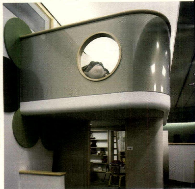
TOP: COMPACT FLUORESCENTS IN A COVE ILLUMINATE THE CURVED WALL OF THE COMPUTER AREA, WHICH IS RAISED TO CREATE A STAGE-LIKE PRESENCE. INCANDESCENT DOWNLIGHTS ACCENT THE COMPUTER SCREENS AND DECORATIVE SCNCES PROVIDE VISUAL INTEREST. DAYLIGHT PENETRATES THE SPACE THROUGH CLERESTORIES ABOVE A PLAY LOFT (RIGHT). A VAULTED CEILING OVER THE LOFT IS HIGHLIGHTED WITH INDIRECT FLUORESCENTS MOUNTED IN A COVE.
