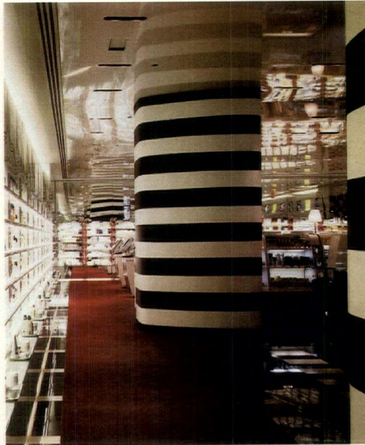
DISPLAYS ALONG THE WALLS ARE ILLUMINATED TO HIGH LEVELS BY ROWS OF FLUORESCENTS CONCEALED IN METAL CYLINDRICAL REFLECTORS.
