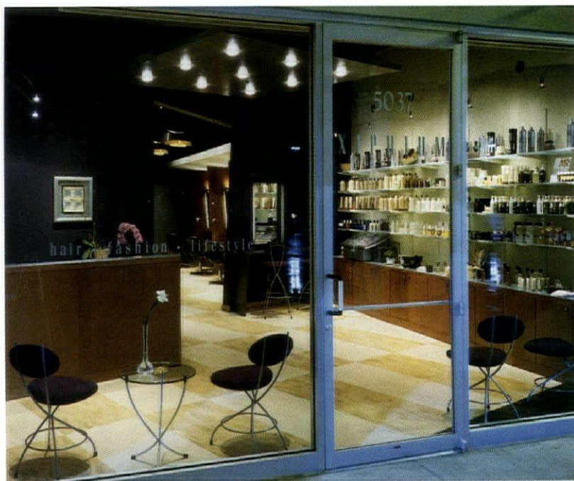
A SERIES OF 50W, LOW-VOLTAGE HALOGEN SOURCES WITH GLASS TRIMS PUNCTUATES A SUSPENDED PLANE OVERHEAD, PROVIDING BOTH AMBIENT ILLUMINATION AND SPARKLING DESIGN DEFINITION TO AN ARCHITECTURAL FORM THAT IS ECHOED OVER THE STYLING STATIONS.
