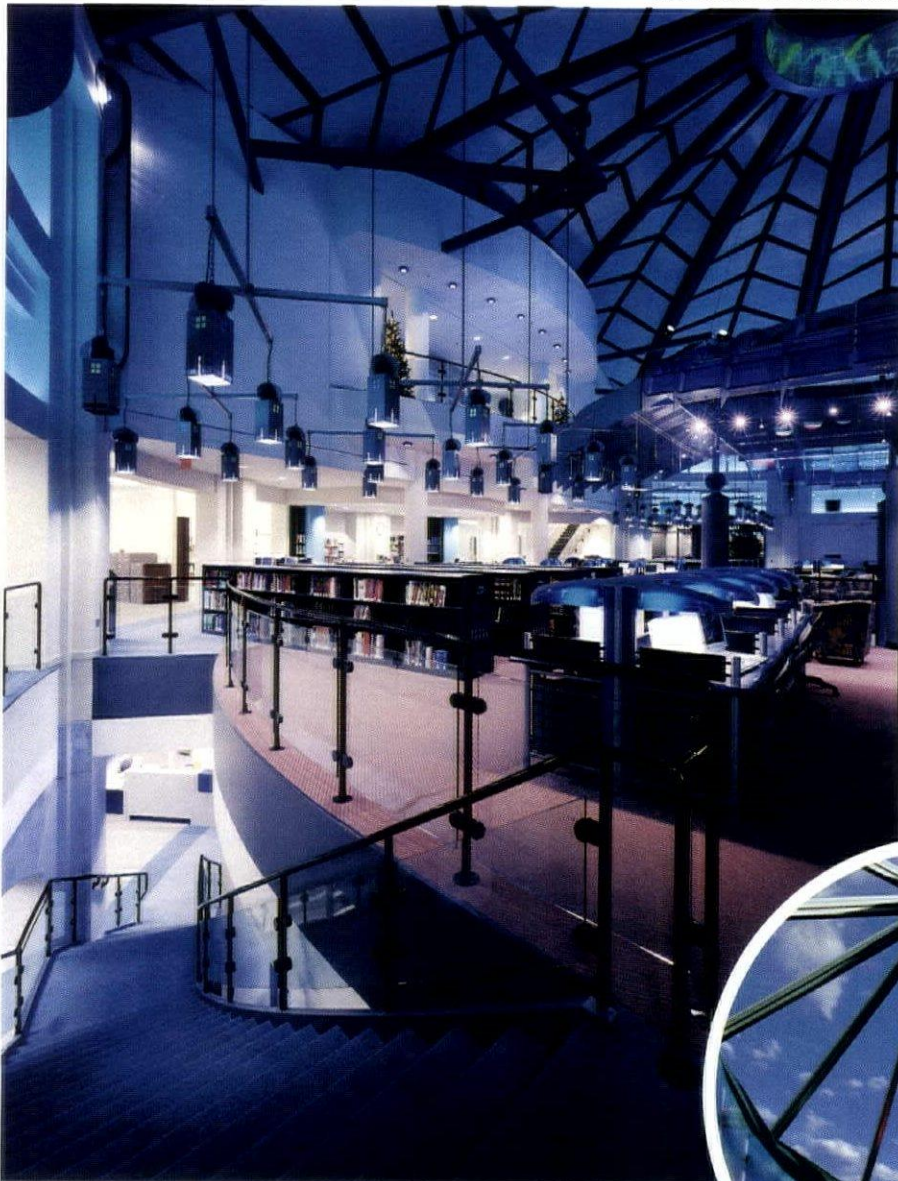
AT THE TOP OF THE LIBRARY'S ROTUNDA, FULLY METALLIZED HOLOGRAPHIC FILM, BONDED TO AN ACRYLIC BACKING AND POSITIONED AROUND THE COLLAR OF THE DOME'S SKYLIGHT, PRODUCES AN ARRAY OF BRILLIANT COLORS WITH REFRACTED LIGHT. TO ADD MORE VISUAL INTEREST TO THE INTERIOR, ROWS OF PENDANT-HUNG METAL LANTERNS, WHICH ILLUMINATE THE AISLES BETWEEN STACKS, FEATURE COLORFUL GLASS ACCENTS.
