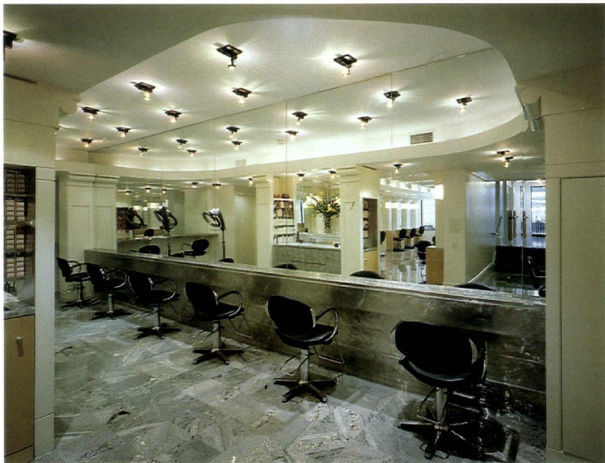
IN THE COLORING AREA, FLUORESCENT COVES OFFER DIFFUSE AMBIENT LIGHT, WHILE ADJUSTABLE HALOGENS WITH A CRI OF ABOUT 100 ARE FITTED WITH BLUE FILTERS TO PROVIDE APPROPRIATE TASK LIGHT THAT SIMULATES DAYLIGHT.
