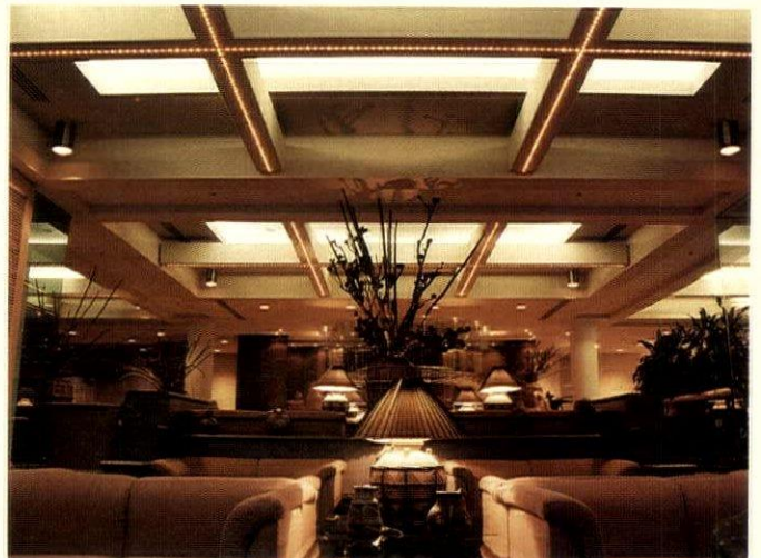
In the Breakers Cocktail Bar, low-voltage tube lighting highlights the ceiling grid.
