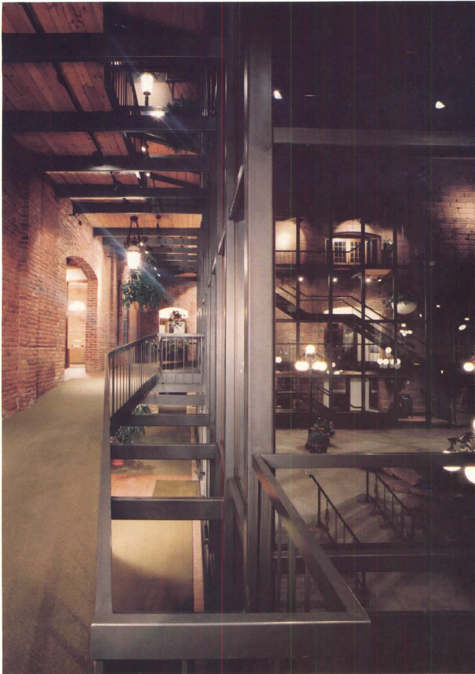
Above, ramps and a glass gallery link the spaces of the Elephant Corral. Openings between the glass and ramps allow circulation of solar-warmed air in the winter. Left, built-in bookcase and level change offer a nook of privacy.
