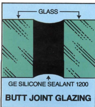
Sealant intended as weather seal only. Not as support or stiffening agent.
