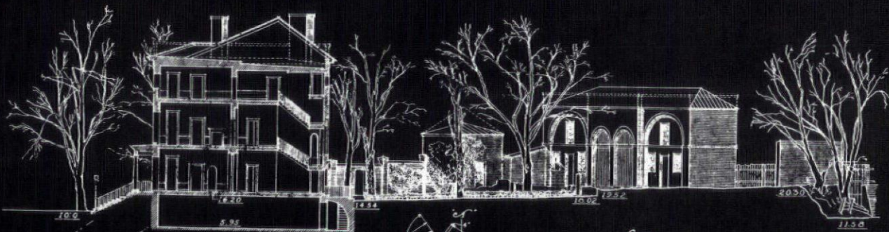
Section: Taken on line 'B' of Plat Dotted lines show supposed original roof treatment.
