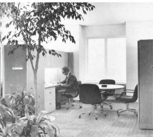
Atlantic Richfield's Philadelphia headquarters office lighting system has served as prototype for T/A illumination. Developed by Sylvan Shemitz, it reportedly delivers 2.56 watts per square foot.
