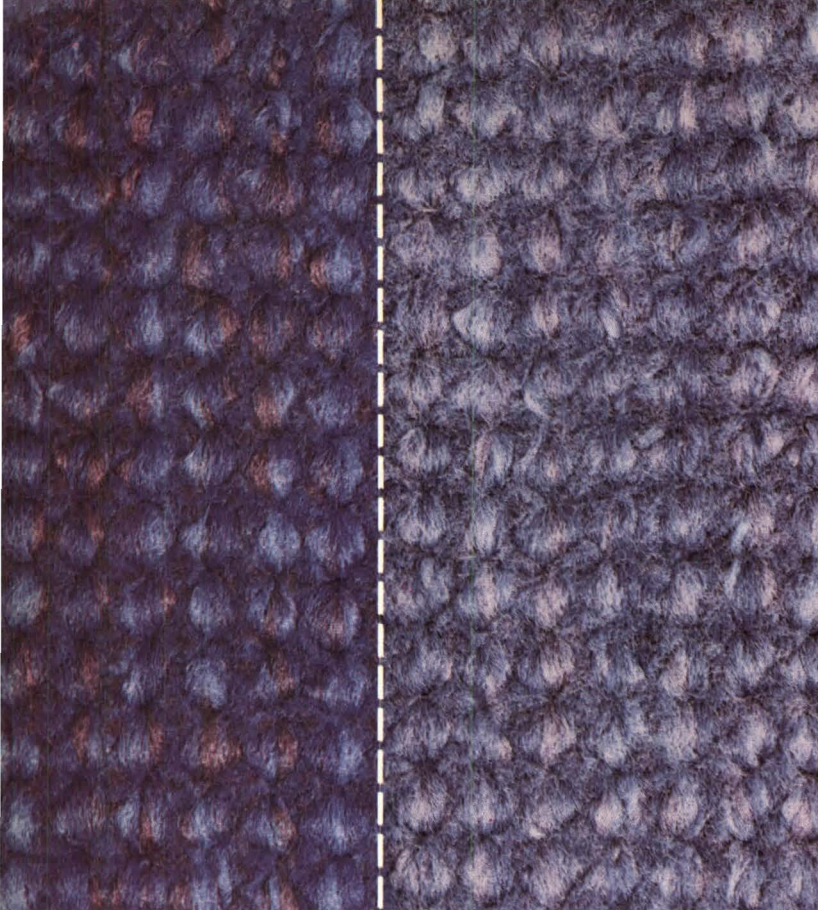
This is how nylon looks before and after exposure to 1500 hours of Xenon-Arc lamps.
