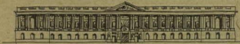
East facade of the Louvre. Gigantic order in a design by Perrault, court physician
