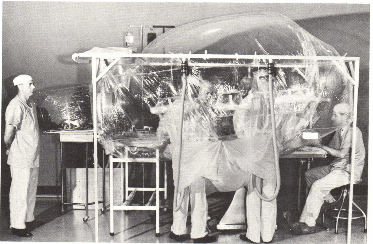
Trexler-Levenson plastic isolation chamber in use at Walter Reed Germfree Laboratory, in a simulated operating room scene. The original surgical tent of this type was developed by Notre Dame University. This design incorporates certain refinements on the original but as yet has been used primarily in animal research
