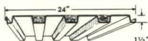
B-ACOUSTIDECK — Two-in-one panel combines steel roof deck with acoustical ceiling having Noise-Reduction Coefficient of .70 — used for spans to 10'0".
