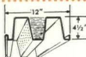
C-ACOUSTIDECK — Offers same Noise-Reduction Coefficient as B-Acoustideck. Can be used for spans to 24'0".
