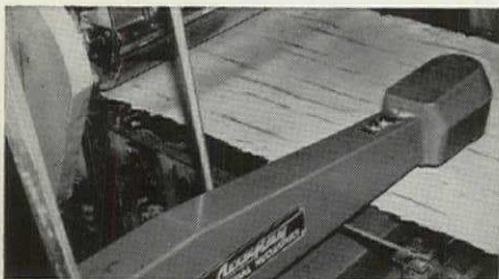
Nuclear gauge continuously inspects tile and controls production processes to achieve desired uniformity. Deviations are corrected instantly.
