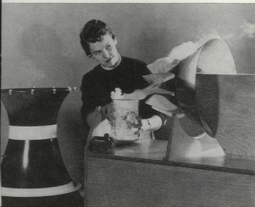
Figure 3. In new type all-plastic fan vanes are mounted perpendicular and parallel to the axis around which they spin, but no spill off or turbulence zone is created. Rotation of bullet-like cone keeps air moving in direct line.
