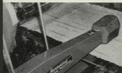
AccuRay clear gauge continuously inspects tile and controls production processes to achieve desired uniformity. Deviations are corrected instantly.
