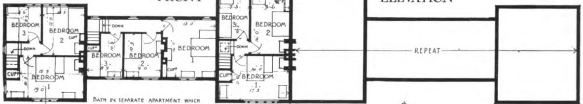
BATH IN SEPARATE APARTMENT WHICH CAN ALSO BE USED AS A WASH HOUSE. BATH CAN BE SUPPLIED WITH HOT WATER FROM COPPER WHEN THE RANGE IS NOT IN USE.
