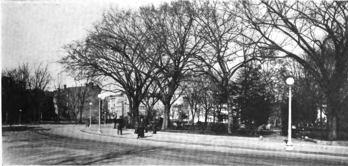
WASHINGTON, D. C., SOUTH SIDE OF DUPONT CIRCLE. Mounting Height of Lights, 12 Feet
