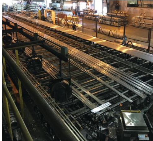
Aluminum billets are pressed through a die to create extruded aluminum shapes or profiles. Following the extrusion process, a variety of options are available to modify the color, texture and brightness of the aluminum's finish.
