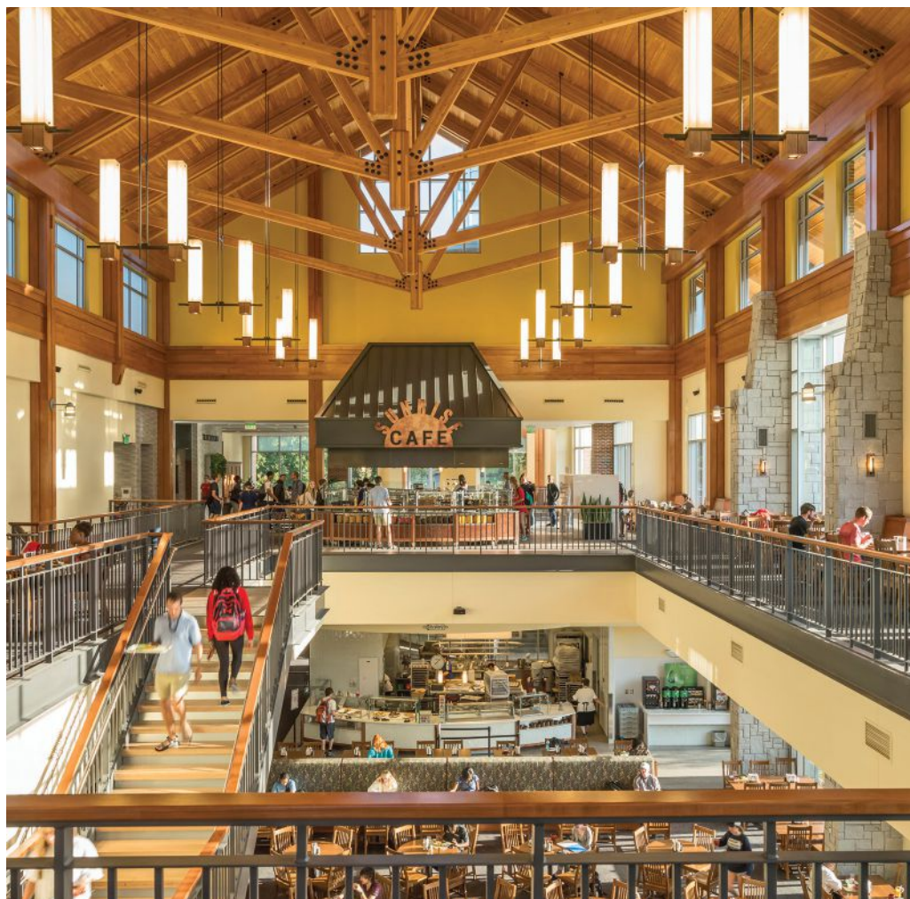
Bolton Dining Commons, University of Georgia | Athens, Georgia | Smith Dalia Architects, Bruner/Cott & Associates In this 50,000-square-foot dining commons, Douglas-fir structural roof decking and truss timbers respond to the client's desire for natural materials that evoke feelings of warmth and comfort, have visually appealing textures and patterns, and resonate with students and staff. Photo by Richard Mandelkorn
