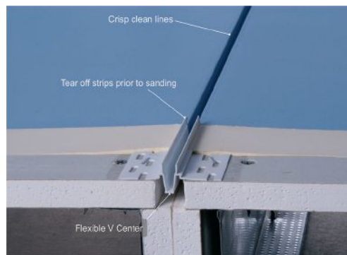
As a general rule control joints should be spaced no more than 30' apart.
