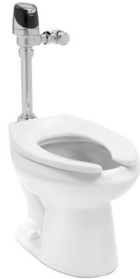
A 1.1 gpf flushometer is only recommended in new construction installations or those where sufficient drain line carry can be assured. Alternatives include 1.28 gpf or 1.6 gpf flushometers. Photo courtesy of Sloan Global Holdings, LLC
