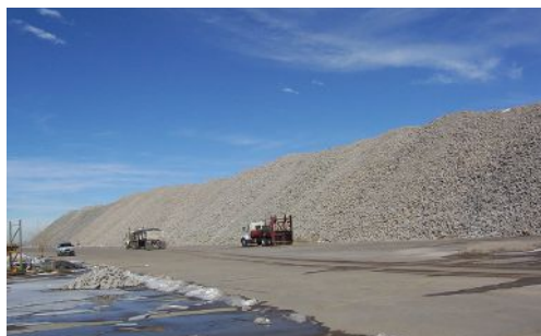
Figure 4—Part of the 6 million tons of recycled concrete generated from runways, taxiways and structures at Denver’s Stapleton Airport—image courtesy of RMCI
