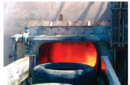
Figure 2—Whole steel belted tires feed into a cement kiln for energy recovery and solid waste reduction.
