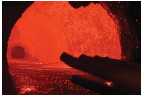
Figure 1—Limestone, silica, alumina and iron chemically combine to form clinker in the rotary kiln of a cement plant.
