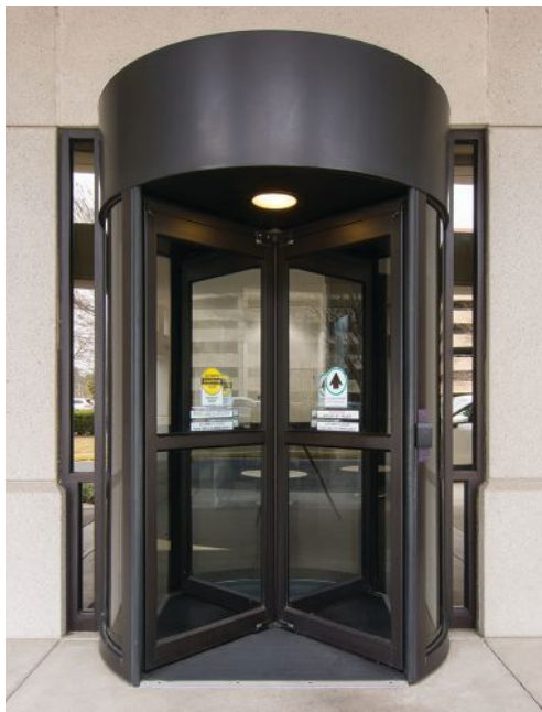
General safety features that are needed to meet building codes and standards include sensors such as a canopy mounted motion detector, a sensor to detect a person in the rotating path, entry point sensors, toe guard sensors, contact safety edges and emergency buttons. Photo courtesy of Horton Automatics
