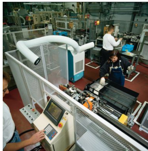
Spot cooling of a small area or process can reduce cycle time, handling damage, reject rates, and increase profits. Photo Credit: MovinCool
