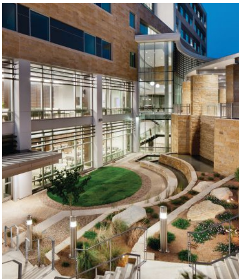
A sunken garden brings a large amount of daylight to lower levels, creates natural views from multiple floors, and aids in wayfinding. Photo Courtesy of Casey Dunn.
