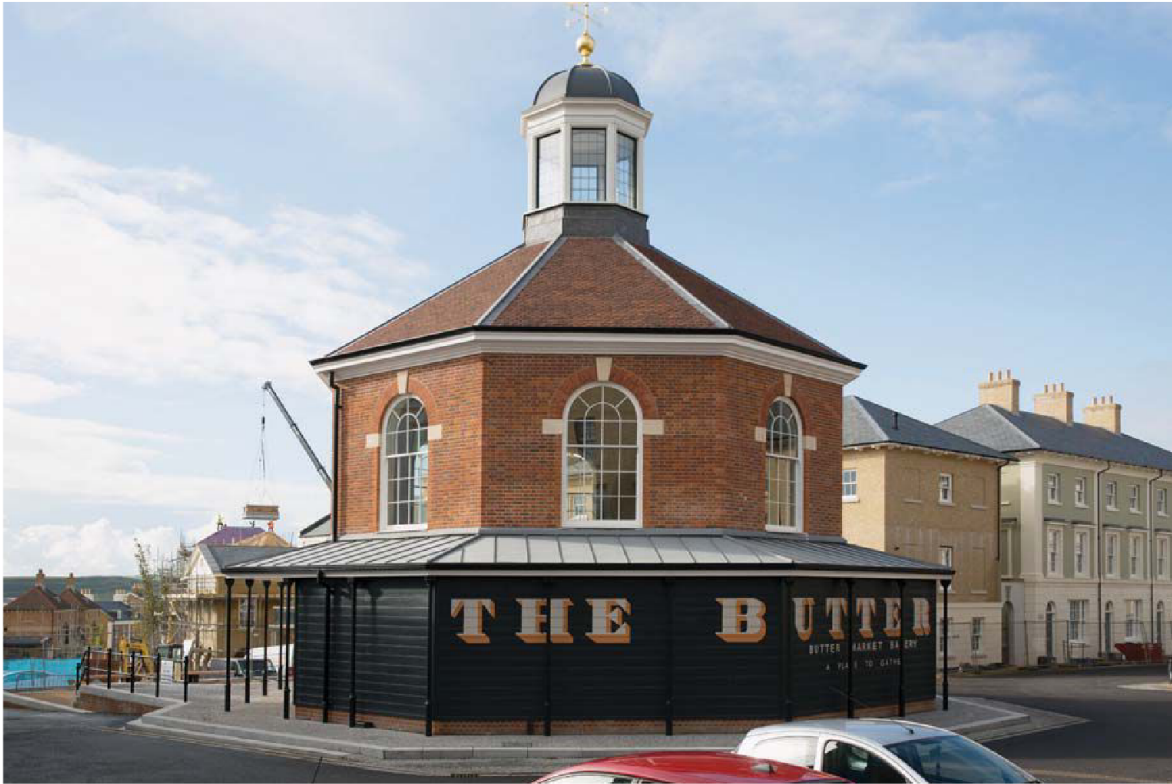
An octagonal building in the middle of Bridport Road, the chief east–west artery through Poundbury, forces drivers to awkwardly skirt the structure—one of many “events” that the town’s planners use to slow the pace of traffic.
