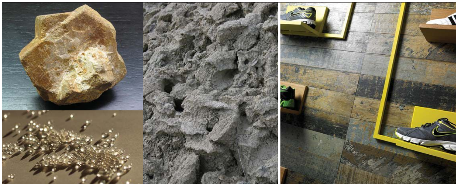
For all its technological innovations, modern ceramics still begin with three basic ingredients: clay (right), sand (bottom left) and feldspar (top left). These ingredients are found in nearly limitless supply on our planet. They are classified as “perpetual resources” and react in a white-hot kiln to create an inert piece of ceramic tile.
