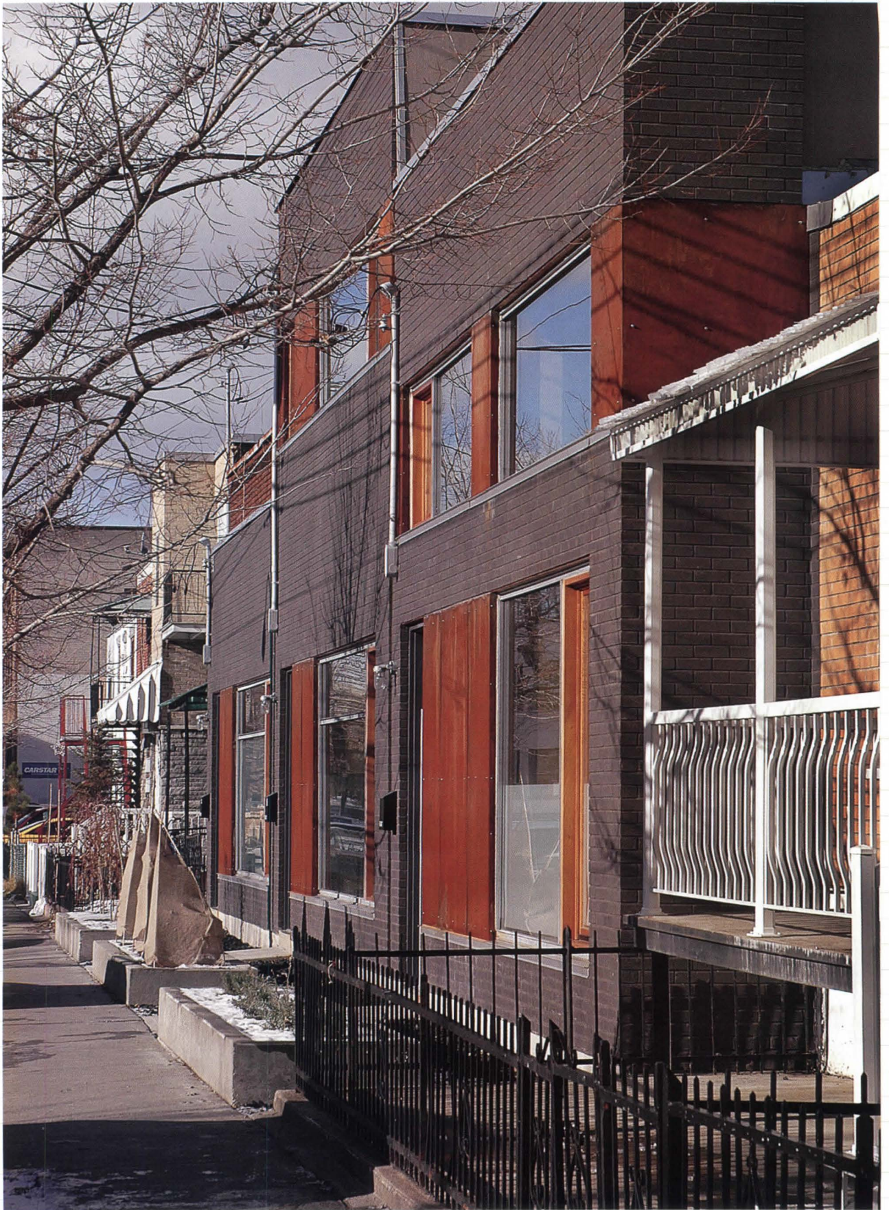
HENRI CLEINGE'S THREE-UNIT TOWNHOUSE GROUPING (ABOVE) IS CLAD IN WEATHERED STEEL, BLACK BRICK, AND STUCCO TO REFLECT THE SEMI-INDUSTRIAL NATURE OF ITS MONTREAL NEIGHBORHOOD. SETBACKS AND VARIED GLAZING MODULATE THE STREET FAÇADE (FACING PAGE).
