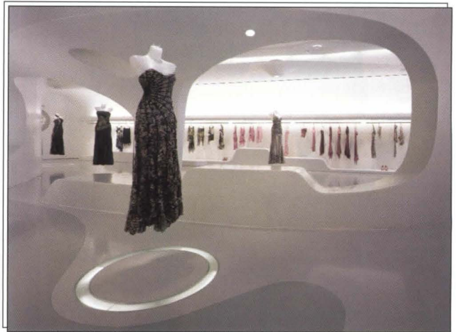
The heat-formed plastic interior of the Carlos Miele store is accented by illuminated floor rings and custom clothing racks with integral light fixtures.
