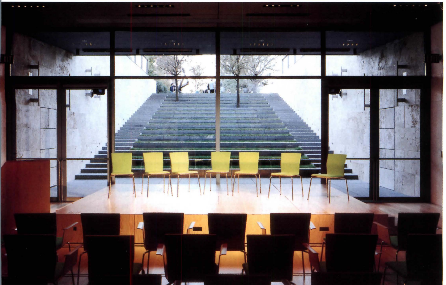
The Nasher's interior walls are clad with 2-inch-thick slabs of travertine, which have been honed to remove the rough outer layers of the stone (above), while exterior walls are coarse and pitted for a weathered finish. Garden and building meet at an indoor-outdoor amphitheater used for both public programs and private events (below).
