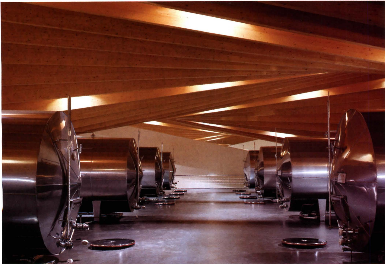
Beneath its roof of rolled cypress beams, the winery's top floor holds 36 stainless-steel tanks, each containing 6,600 gallons of wine.
