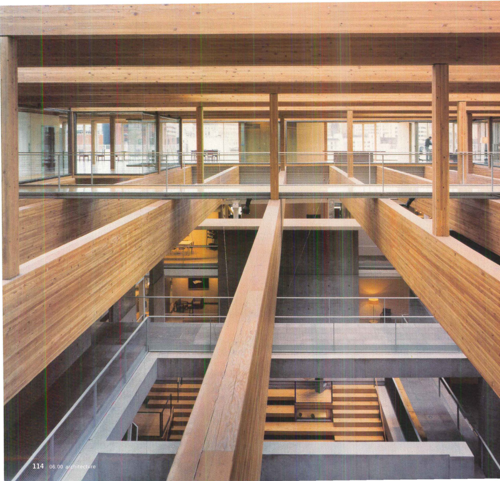
A complex series of bridges and stairways leads up to and through the atrium space (above). A penthouse floor (below) sits above the atrium, on giant glulam beams. A terrace outside the penthouse (facing page) overlooks downtown Portland.
