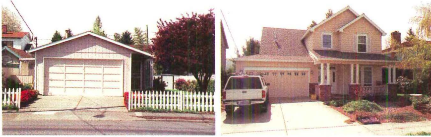
“Snout” house gives neighbors only garage views (far left); alternative scheme (left) preserves garage and street-side friendliness.
