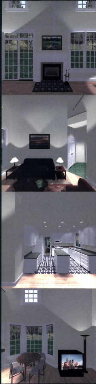
Unwrapped QuickTime VR image (facing page) demonstrates how individual rendered images are joined to form 360-degree scene. Walk-throughs produced with QuickTime VR (above and right) permit movement through virtual architectural environment and views from any angle and position in room.
