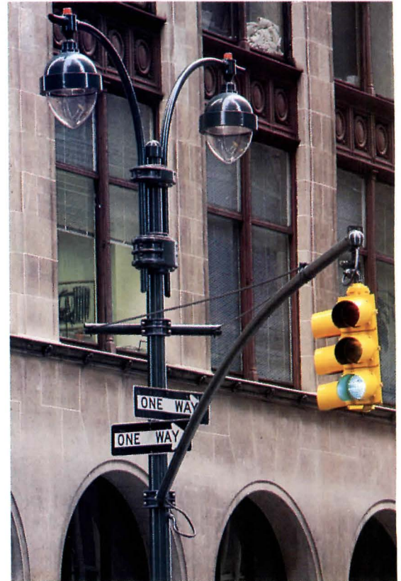
ACORN HEAD: Metal halides replace high-pressure sodium lamps.
