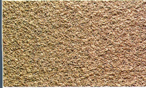
Light Dash: A first coat is dashed for complete color coverage. When it dries, a second coat of thinner consistency is dashed or sprayed on with an atomizing gun.
