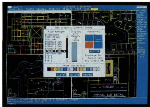
The Nth Drive display-list-processing software for AutoCad 386 shows the Nth Engine's control panel (above). The Nth Engine/150 supports 256 colors at a resolution of 1,280 by 1,024.
