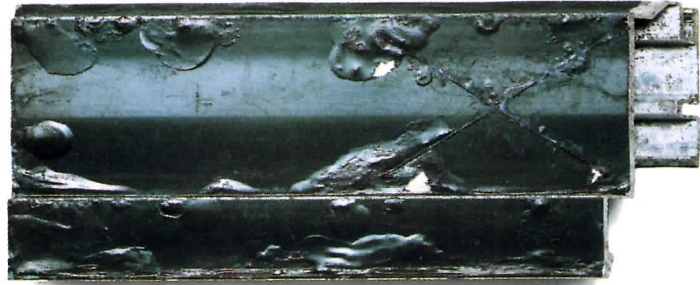
Ordinary paint, after the equivalent of 3,000 hours of 5% salt fog. (AAMA 605.2)
